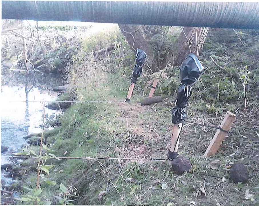
Figure 2.3: Pair of PIT antennae shown with support structures. Tuning boxes were housed in black plastic for protection. Photograph taken on 24/09/2014.
