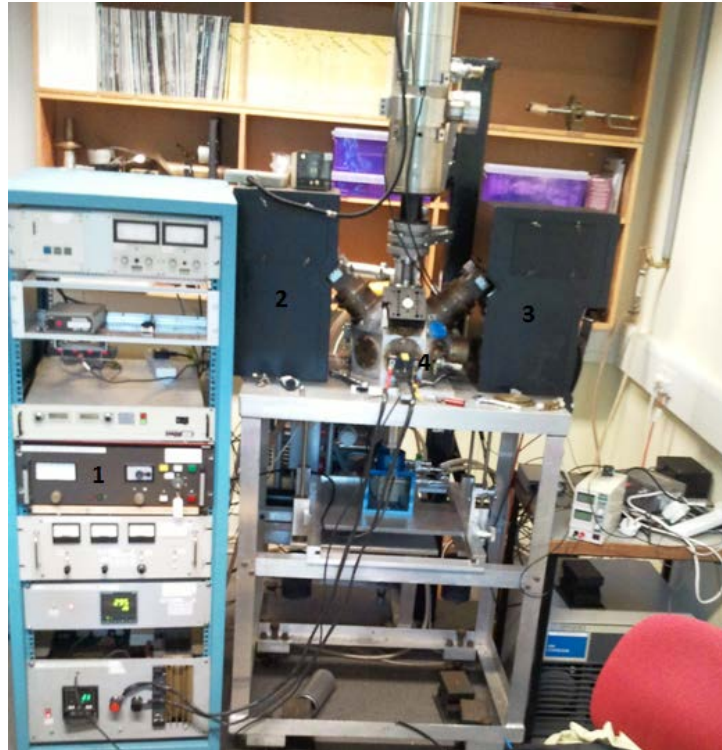
Figure 5.5: Photograph of the RL/TL system at the Facility for the Luminescence of Minerals at the University of St Andrews. The basic components of the instrument are (1) power supply of x-ray generator emitting Cu Ka x-rays, (2) UV-blue (250-550 nm) spectrometer (3) blue-green-red (380-850 nm) spectrometer, (4) cryogenic sample holder. Courtesy of Dr Adrian Finch.
