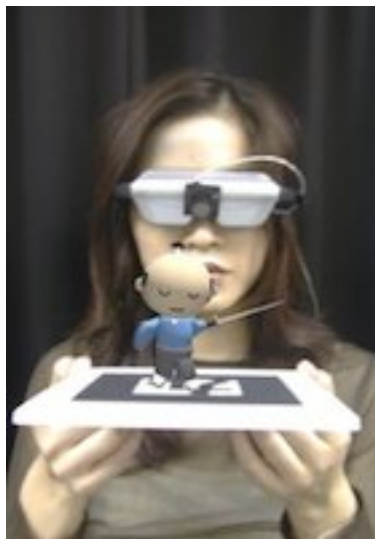
Figure 2.3: Example content attached to a marker in ARToolkit (Kato and Billinghurst (1999))
