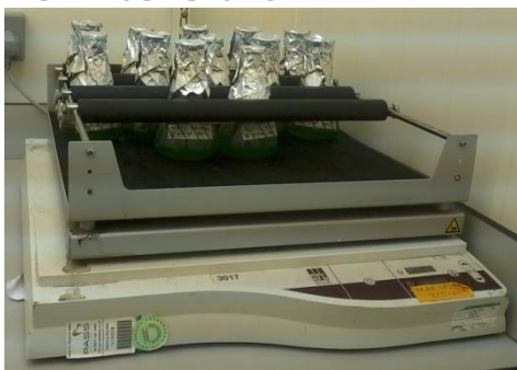
Figure 6: Arrangement of flasks containing Scenedesmus obliquus on KS501 Digital IKA Labortechnik flask shaker in growth room used in this study.
