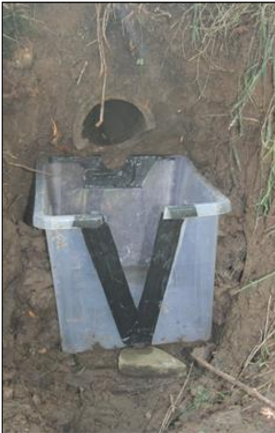
Figure 4.5. The shallow groundwater monitoring weir
