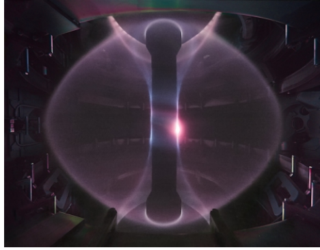
Figure 1.7: Colour photograph of a plasma inside the MAST vessel. Deuterium Balmer-alpha ( D_\alpha ) emission at 656.1 nm dominates the visible part of the spectrum. Also visible in the image are in-vessel poloidal field coils (top and bottom) and smaller radial coils (bottom left and bottom right) used to perturb the edge of the plasma to control the MHD stability of the edge region. The bright spot on the centre column marks the location of a gas valve used to fuel the plasma; emission from the injected gas can be seen wrapping around the centre column in the middle of the image as the fuel becomes ionised and starts to flow along the field lines.. Image credit: Dr. Scott Silburn and Dr. James Harrison.
