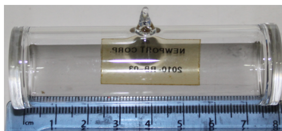
Figure 4.1: A vapour cell containing rubidium. The internal distance between the windows is 75 mm.
