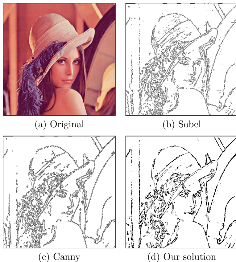
Figure 5.5: A comparison of final edge maps produced by the Sobel, Canny and our parallel ACO edge detection algorithms.
