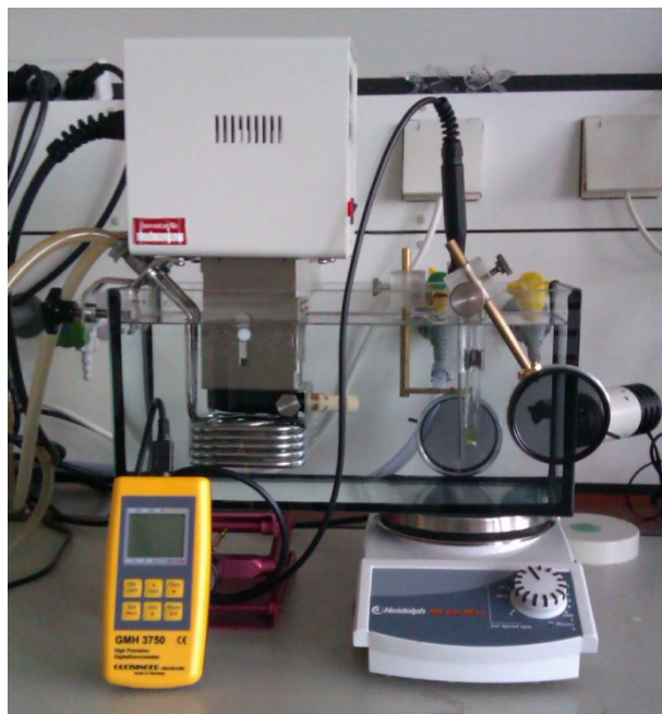
Figure 6.1: Water basin used to determine the phase boundaries of a microemulsion. It is equipped with a thermostat with attached tap water cooling, a magnetic stirrer, a sample holder, a digital thermometer, a lamp and crossed polarisers.
