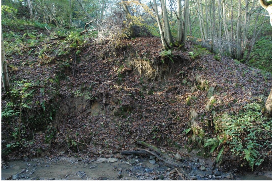
Figure 5.9-Photo demonstrating the geology and high amount of vegetation on the monitored landslide face taken in October. The landslide face is approximately 10 m high by 10 m in length.
