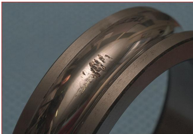
Figure 6.8: An example bearing race suffering from surface fatigue of the inner race Stevens (2011).
