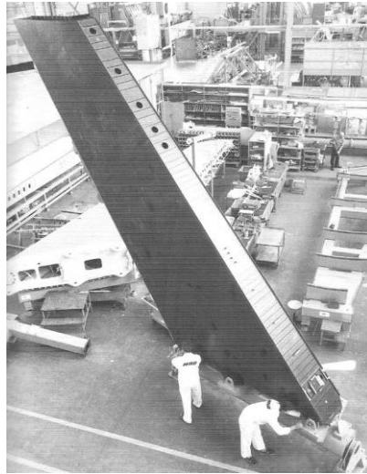
Fig.1.12 All-carbonfibre reinforced plastic fin box of Airbus A310 From Whitford 'Structure and Materials' p.79
