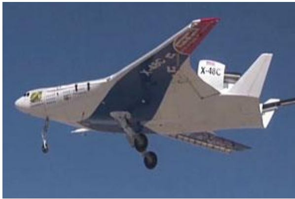
Fig.1.15 X-48C Blended Wing Body Test Model Aircraft (From www.boeing.com/Features/2013/04/bds_x48c_04_24_13.html )
