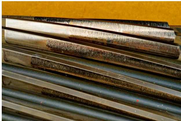
Figure 6.5: HSS pinion damage on the NREL 750 kW gearbox, photograph from GEARTECH/NREL 19743.
