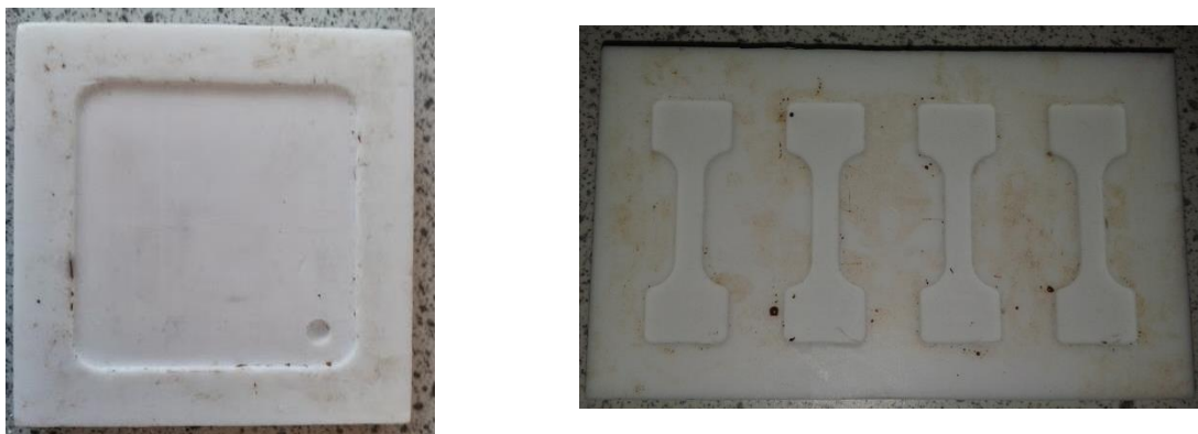
Figure 6.5 – (Left) Standard PTFE mould, (right) mould for DMA
