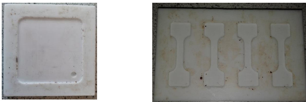
Figure 4.28 – PTFE moulds for producing samples of approximately 1 mm. (Left) mould for most analysis; (Right) mould for thermo mechanical analysis.
