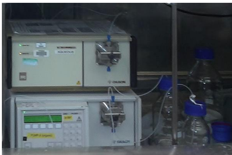
Figure 6.3 – HPLC pump set up. Bottom is a Gilson 305 pump with system control set for aqueous solvent. Top is a Gilson 306 as the secondary pump set for organic solvent.
