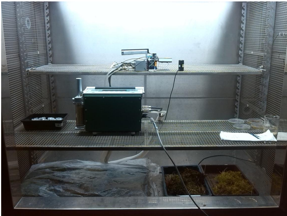
Figure 5: LI-COR photosynthesis system set up with bryophyte chamber inside the climate controlled chamber.
