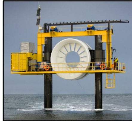
OpenHydro Open-Centre Turbine
