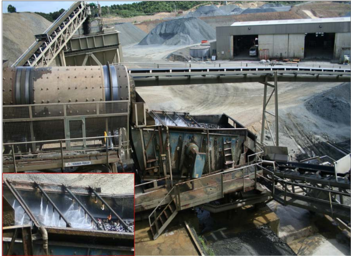
Figure 6.1 Water sprays over the processor at Hanua quarry, New Zealand, inset: magnification of sprays featured in central portion of the main photograph.
