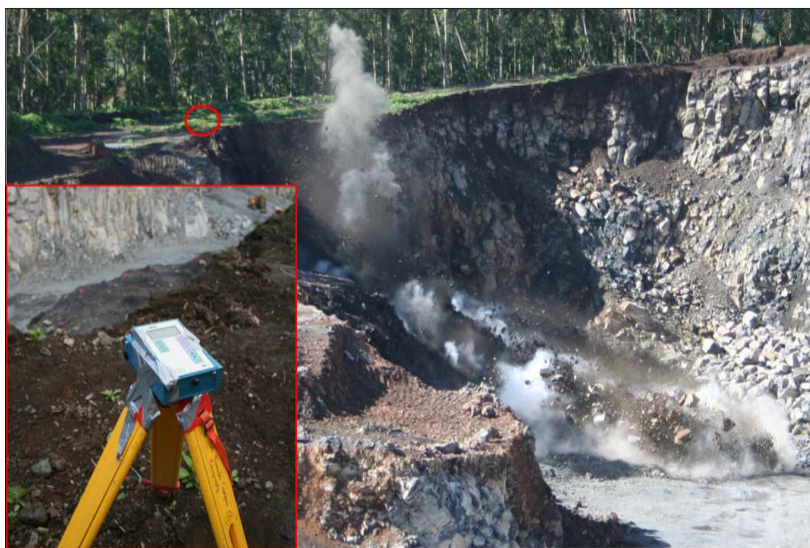
Figure 6.3 DustTrak location during a blast at Bombay quarry, New Zealand (location of DustTrak indicated by red circle). inset: looking down onto the blast site (prior to blasting) from the DustTrak location. The explosives can just be seen in the midground (indicated by bright pink dots on dark grey surface).
