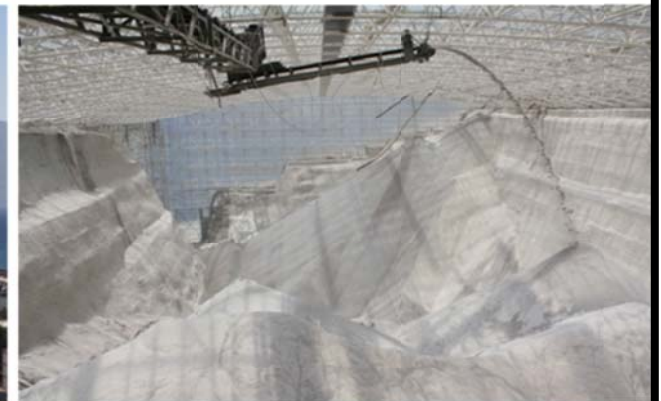
Stockpiled perlite is kept in a plastic hangar to prevent contact with rain.
