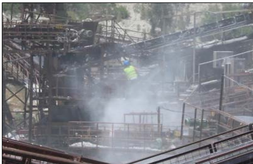
Figure 6.21 A worker at LAVA pumice quarry climbs to an upper platform on the processor to shovel a mound of dust from it whilst stood in a visible dust cloud. He was not wearing any respiratory protection.
