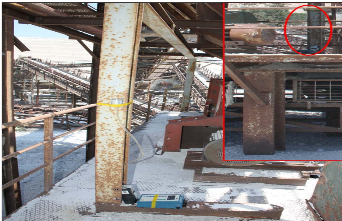
Figure 6.8 DustTrak and Sioutas on the processor at LAVA quarry, Yali. The instruments were always mounted at adult breathing level (1.5-2m off the ground). Inset: positioning of instruments on processor platform, but in breathing zone of the path next to the processor.
