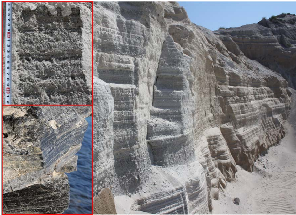
Figure 3.13 The perlite deposit at Aegean Perlite quarry, Yali islet, Greece. Top inset: an area of quarry wall with outer layer removed, to ensure sampling is of material with a fresher surface (scale in cm). Bottom inset: a section of the obsidian dome
