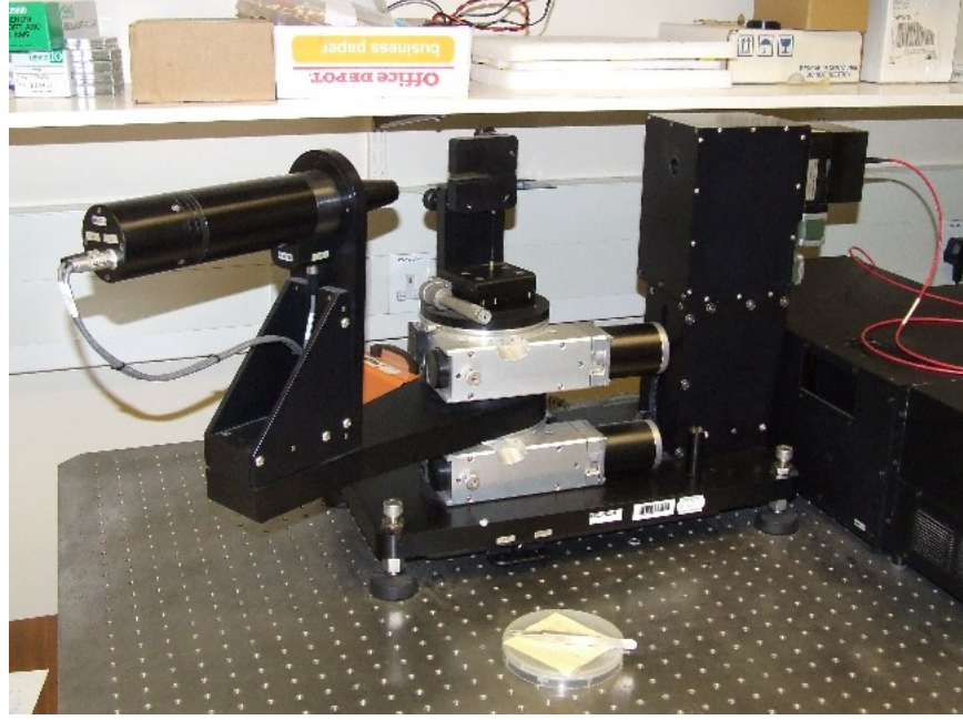
Figure 3.17: Photograph of the J A Woollam VASE ellipsometer used for thin film thickness measurements.
