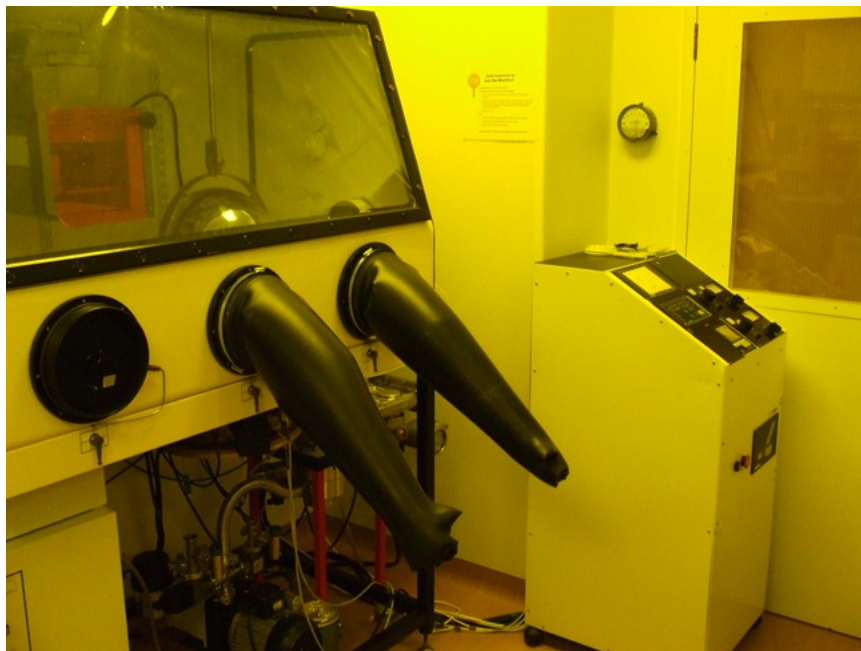
Figure 3.4: Photograph of the Edwards metal evaporator used to deposit the cathode. The evaporation bell jar can be seen in the right hand side of the glove box, while the control unit is outside the glove box on the far right.
