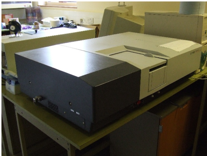
Figure 3.13: Photograph of the Shimadzu UV-3600 UV-VIS-NIR spectrophotometer used to measure absorption spectra.
