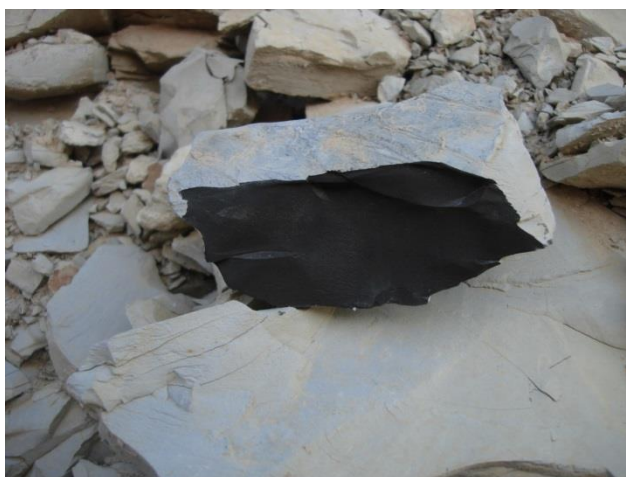
Figure 3.5 - Photo showing the cross section of a piece of oil shale from the Al Lajjun deposit, Jordan.
