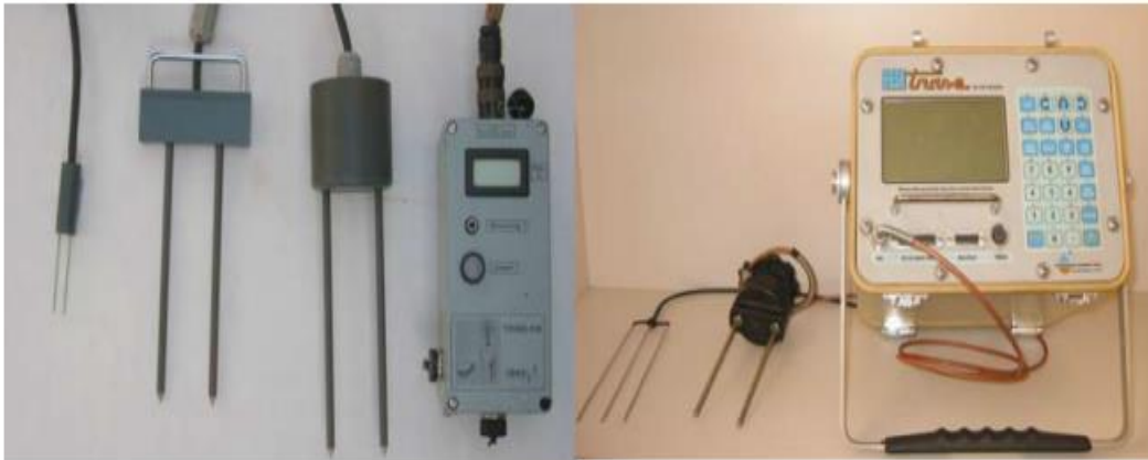
Figure 2.5. TDR probes (Muñoz-Carpena et al., 2006)
