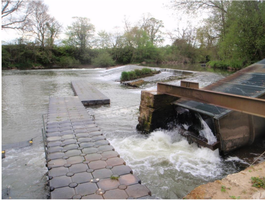
Figure 2.4 Floating pontoons located downstream of the weir and the turbine showing some drift nets deployed below the turbine.
