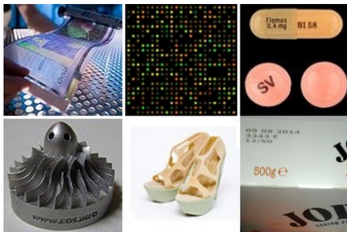
Figure 1.4. Examples of inkjet applications, including a flexible display (from [38]), a microassay of DNA (from [39]), printed labels on pharmaceutical tablets (adapted from [40] and [41]), a 3D mock-up of a turbine (from [42]), 3D-printed shoes (from [43]), and packaging labels.
