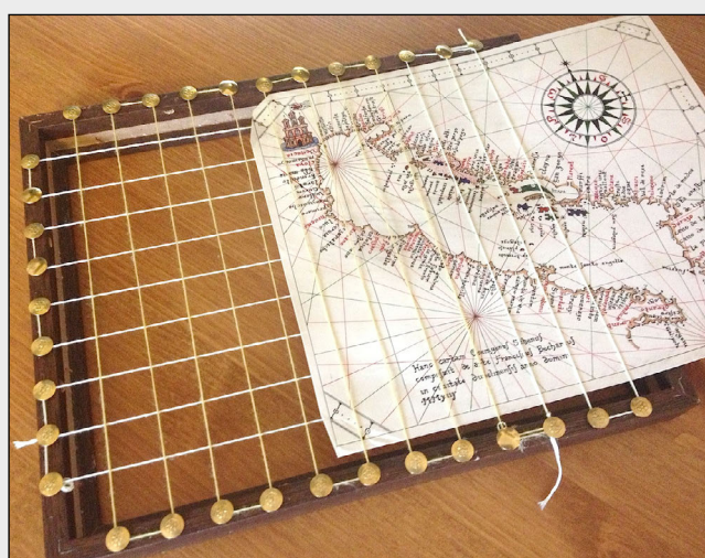
Figure 1.25: An example of a scaled-down frame described by Bartolomeo Crescentio. The second reconstructed map is shown sliding between the perpendicular strings.
