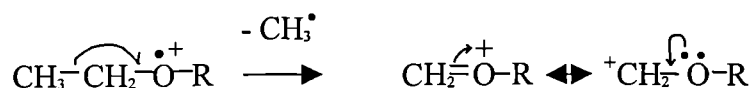
Figure 5.2.5: Fragmentation in EI mass spectrometry of ethers due to cleavage of the C-C bond next to the oxygen atom.
