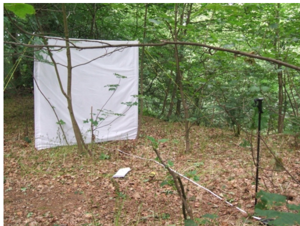
Figure 5-2. Photograph showing equipment layout for measuring vegetation density.
