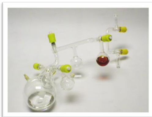
Figure 4.29 "christmas tree" reaction vessel for living anionic polymerisation.
