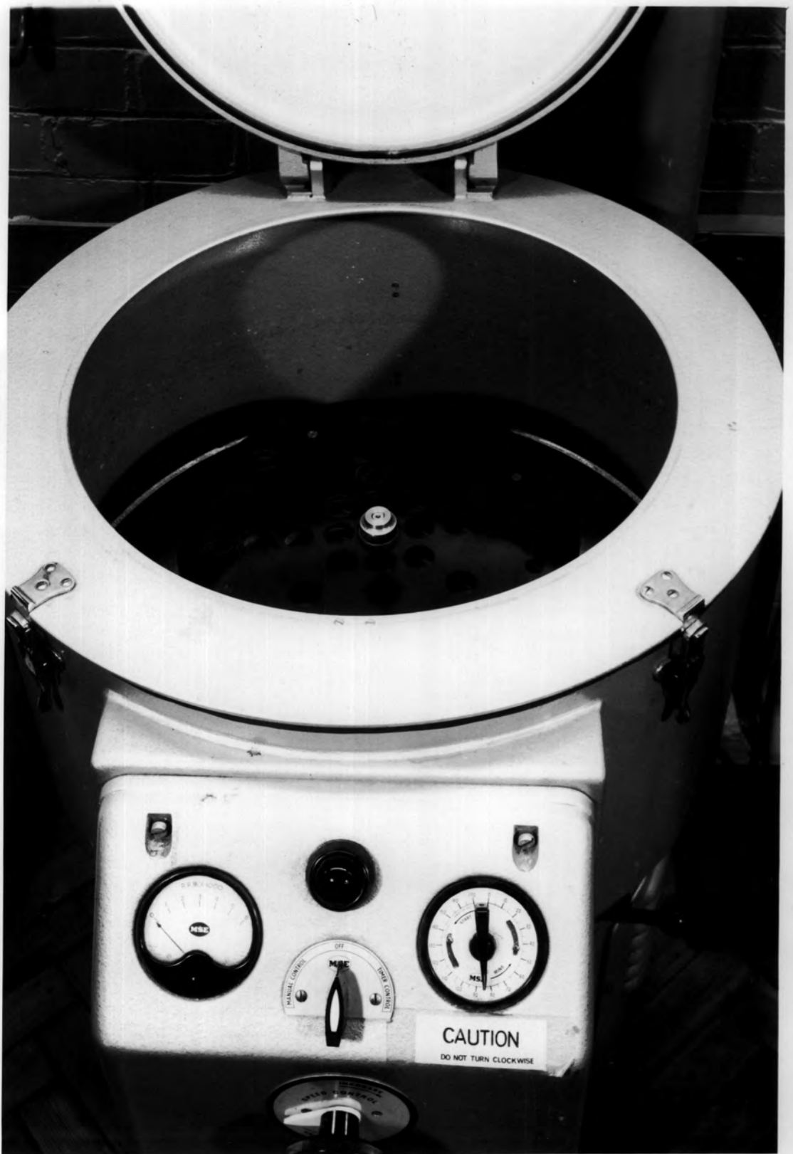
Fig. 4 MSE centrifuge with turntable made to take oxid cap. culture vessels.
