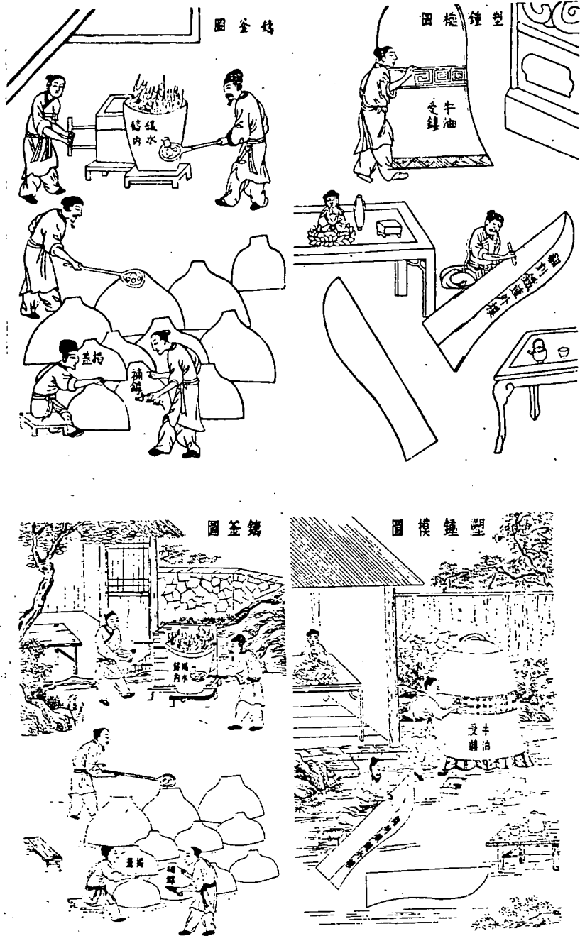
Plate Six. "Preparation of the wax model and the casting of pots and pans. The two scenes are from iron foundries, but are representative of identical procedures in the casting of bronzes; the artisan (upper right) is engraving designs in the wax coating covering a bell core; below, another man is at work touching up the décor of the outer mould-sections." ( Bronze Casting , pp.102-3.) The
