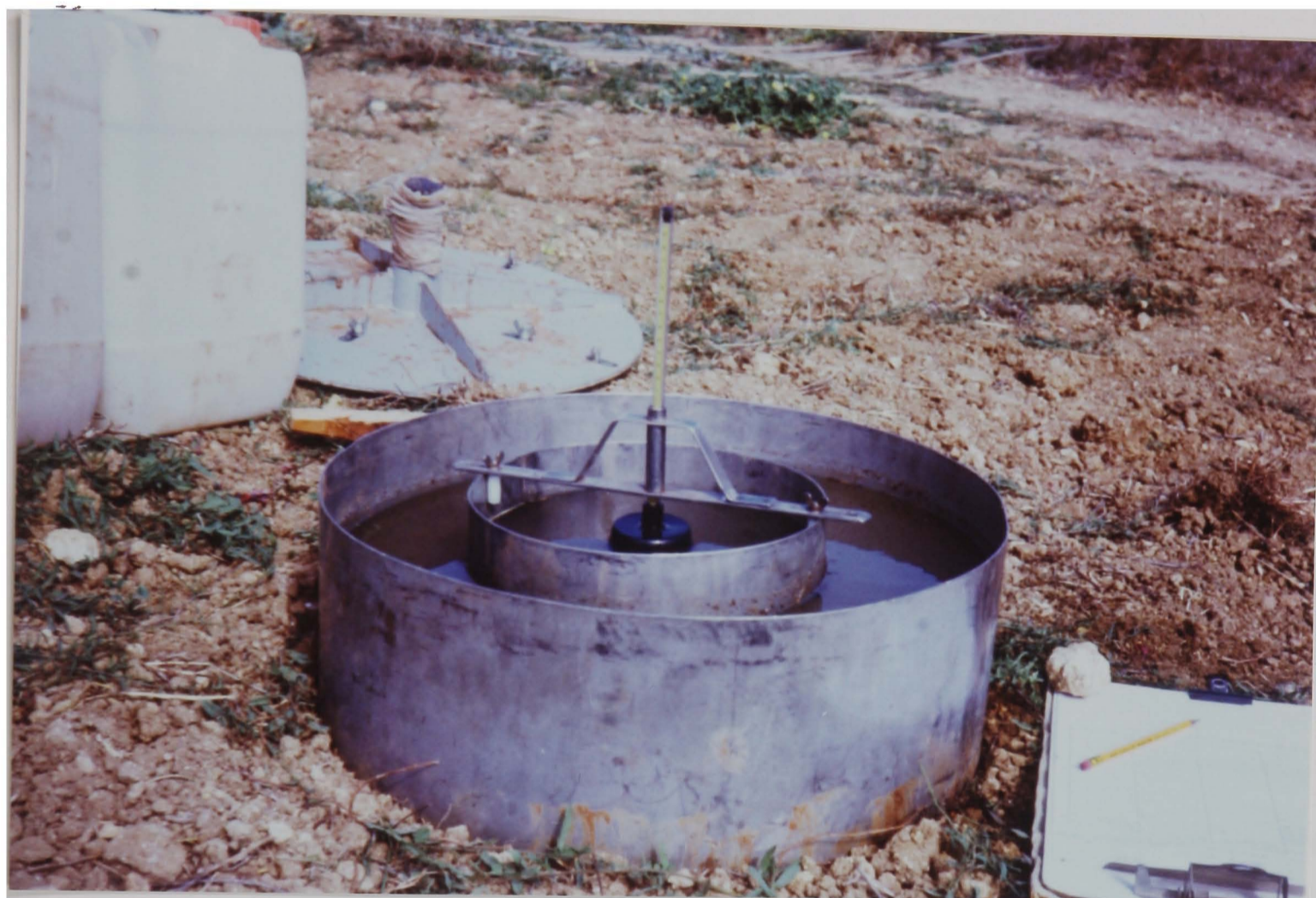
Plate 4.3 Measuring infiltration rate by double cylinder ring.
