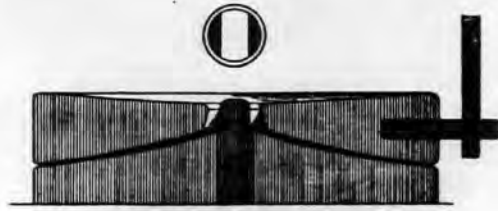
Fig. 81. Section of a Roman hand-quern from stones found at Silchester. ( \frac{1}{4} linear.)
