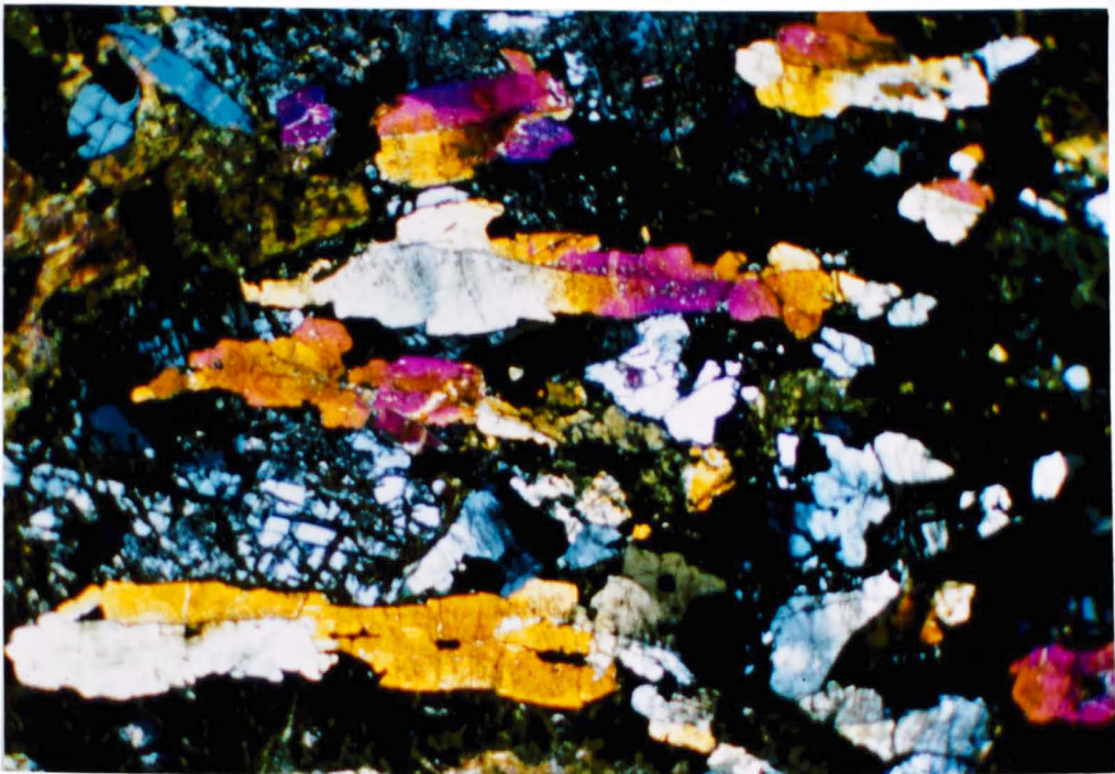
PLATE 4.10b Photomicrograph : Elongated augite showing 'corkscrew growth' phenomena, in subunit B2. (135, XP. Width of field - 8 mm).
